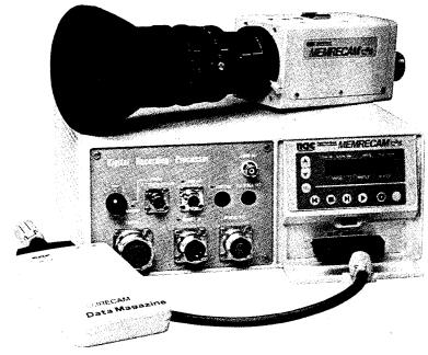
The processor holds the system circuitry, interface circuitry, and digital memory that records up to 80 seconds of images. The unit's small size and light weight make the unit easy and convenient.
